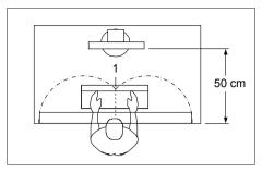
Position the monitor so that the eye distance to the screen (1) is around 50 cm.
