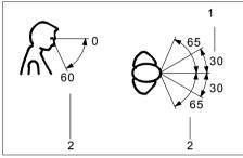
► Position the monitor for optimum viewing (1). The monitor should under no circumstances fall outside the permissible viewing space (2).
