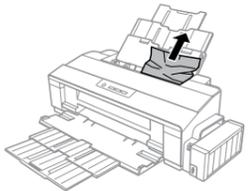
Close the printer cover. If the jammed paper remains near the rear paper feed, carefully remove the paper.
