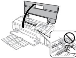
Open the printer cover and remove all of the paper inside, including any torn pieces.
