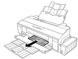
If the jammed paper remains inside the output tray, carefully remove the paper.
