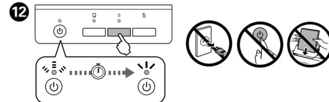
Press  $\Delta$  for 3 seconds until  $\Delta$  starts flashing. Charging ink takes about 22 minutes. Wait until the light stays on.
