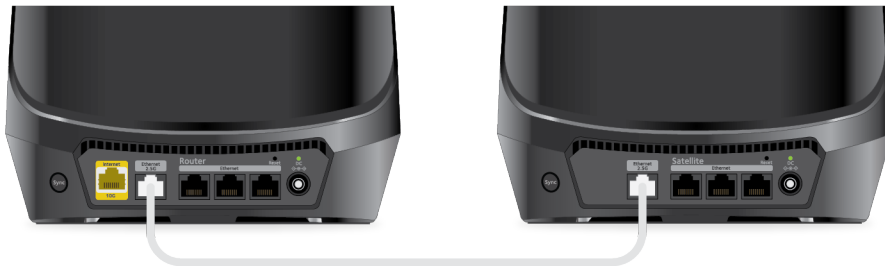
Figure 3. Satellite 2.5G Ethernet port connected to the router 2.5G Ethernet port
