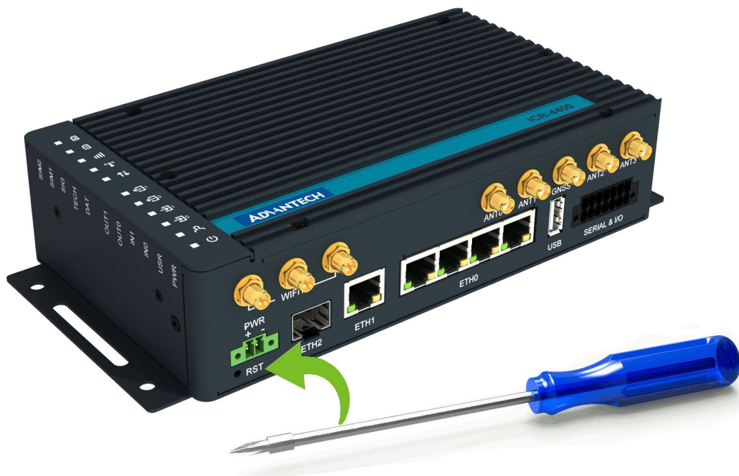
Figure 23: Resetting the Router
