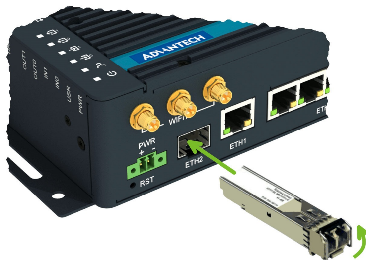
Figure 15: SFP Module Installation
