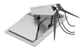
NOTE: Ensure that the cables may pass through the bottom of the cable cover.
