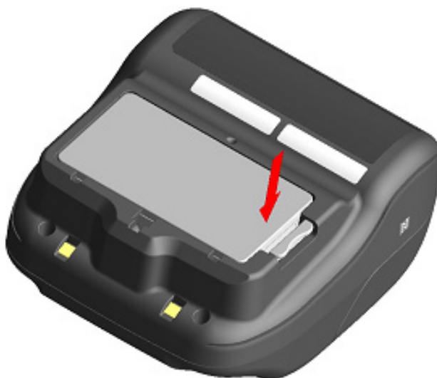
Figure 8-3 Installing Battery Pack (2)
