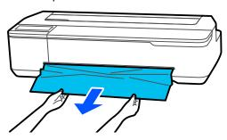
Open the front cover, remove the jammed paper, then close the front cover.
