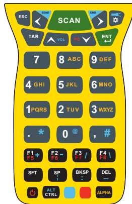
34-Key Numeric (Calculator) Keyboard
