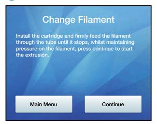
You will then be asked if a filament cartridge is already installed. Initially this will be 'No' as this is the first time a filament cartridge has been loaded; but when changing a cartridge in future you will select 'Yes'. Selecting 'Yes' will uninstall the existing filament before allowing you to load a new filament.
