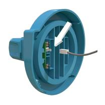
Set up the filament holder cable:
