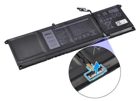
CAUTION: DO NOT pull the battery cable to disconnect it from the battery. This may damage the battery or the battery cable.
