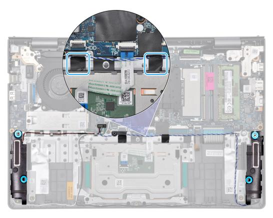
4. Connect the speaker cable to the connector on the system board.
