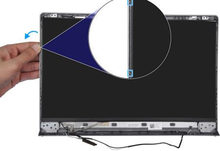
5. Lift the bottom side of the display panel and slide it downward to release the display brackets from the slots at the top side of the display cover.
