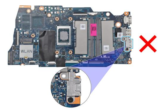
5. Carefully lift and remove the system board from the palm-rest and keyboard assembly.
