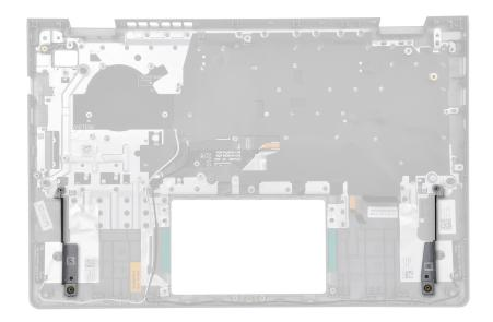
**3.** For computers shipped with an aluminum chassis and a 3-cell battery installed, replace the two screws (M2x2) to secure the left RF metal wall bracket to the palm-rest and keyboard assembly.
