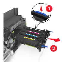
**8** Remove the used developer unit.
