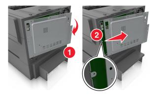
**4** Locate the appropriate connector on the controller board.
