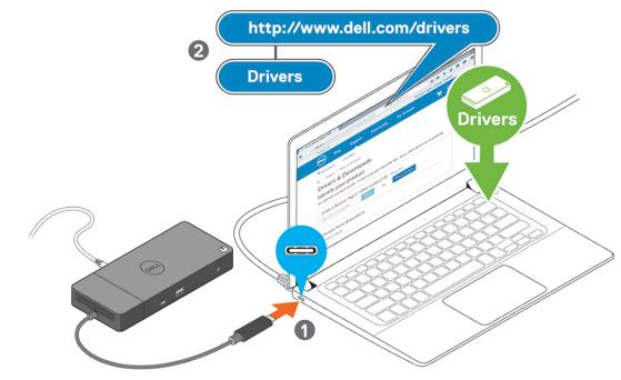
Figure 7. Connecting the USB Type-C connector
