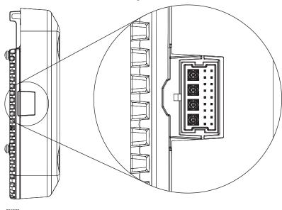
Figure 5 Smart Antenna Connector on the Right Side of the 2802E Model
