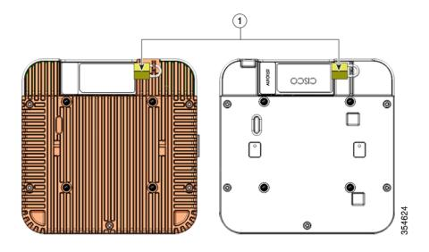
1 Position of the hasps for the locks on the back of the 2802I and 2802E models
