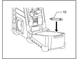
Install the soft bended rod antenna as shown in the figure.
