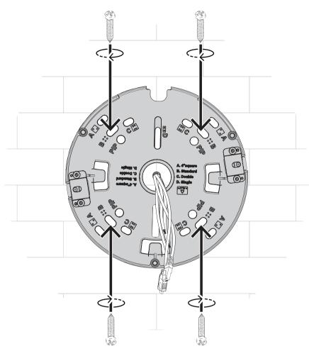
In order to ensure proper wall installation with the Bosch logo showing up straight on top, the mounting plate needs to be install as shown above.
