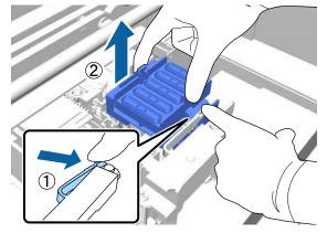
Attach the cover removed in step 7 to the old anti-drying cap, and then put it into the bag of the new anti-drying cap.
