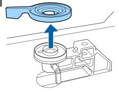
Change the status of the spacer in step 4 according to the installed platen and the thickness of the fabric to be printed on.
