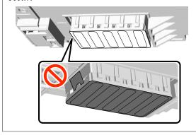
(1) Wipe the edges at the front and rear of the nozzle surface.
