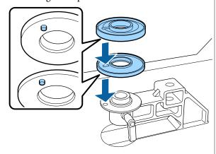
Install the platen gap adjustment lever in the direction shown below.
