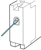
Make sure that the supply port is free of dust when storing cartridges. The port does not need to be capped since there is a valve inside.
