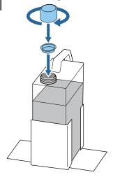
Remove the used waste ink bottle from the waste ink bottle holder, and then insert the new bottle.
