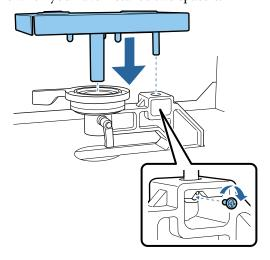
Tighten the fixing lever to secure the platen gap adjustment lever.
