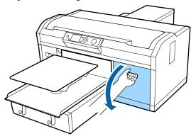
Put your finger into the indentation on top of the ink cartridge to be replaced, and pull it straight
