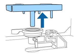
Remove the platen gap adjustment lever.
