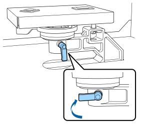
Make sure the axes of the replacement platen fit into the holes.
