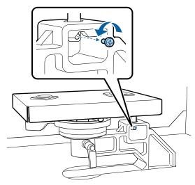
Remove the platen installation plate.
