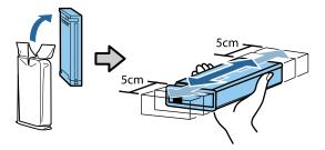
Match the color of the cartridge to the color of the label on the printer and insert.
