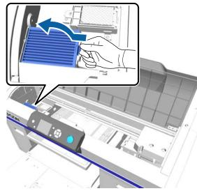
Put the old air filter into the bag of the new air filter.
