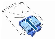
Press the lever forwards, and then place the holes in the anti-drying cap over the two poles on the printer.
