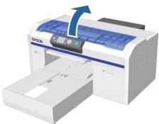
Remove the protective cover, and then press the OK button.
