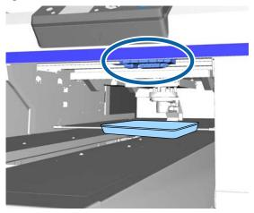
Look into the print head from below the control panel, and wipe off any ink deposits, lint, and dust from the parts that are indicated in the illustration.
