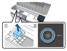
7 Install the charging unit, and then press the OK button.
