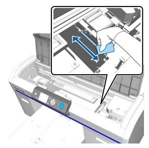
Wipe the border of the metal on the right of the flushing pad.
