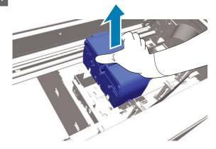
To avoid soiling your surroundings with ink, wrap the used wiper unit in the packaging supplied with the new wiper unit.
