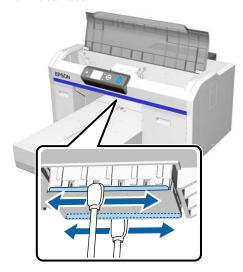
(2) Wipe the parts on the left and right of the nozzle surface.
