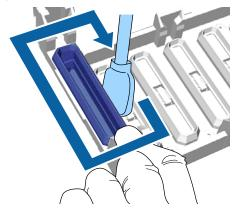
When wiping the outside of the suction cap, remember to also wipe the top edge.
