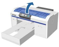
Place your fingers in the groove on the back of the wiper unit, and tilt it forward a little.
