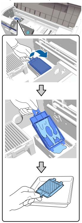
Place the removed flushing pad in the packaging that contained the new flushing pad.
