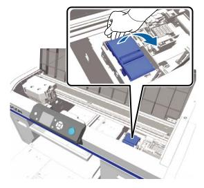
Grip the sides, and pull it straight up to lift it out.
