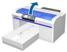
After the print head has moved to the maintenance position, place a metal or plastic tray, or paper under the print head.
