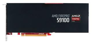
Compute-intensive workloads are no challenge for AMD FirePro S9100 server GPUs. With support for OpenCL, 12GB GDDR5 memory and ECC memory support, up to 2.11 TFLOPS of peak double-precision floating-point performance and up to 9.4 GFLOPS per-watt peak double precision performance, it's clear the AMD FirePro S9100 is a high-performance computing powerhouse.
