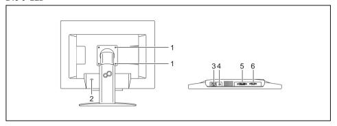
1 = Holes for fixing swivel arm or wall bracket
