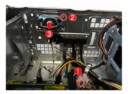
To replace the speaker, reverse the removal procedures.
