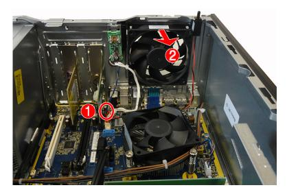
To install the fan assembly, reverse the removal procedure. Be sure to orient the air flow out of the unit.
