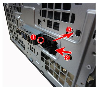
5. Remove the cables from the clips on the base pan.
