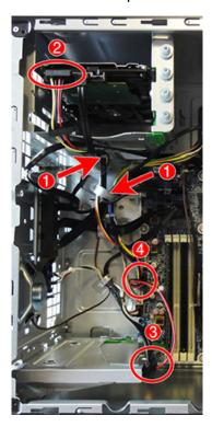
To reinstall the drive power cable, reverse the removal procedure.
