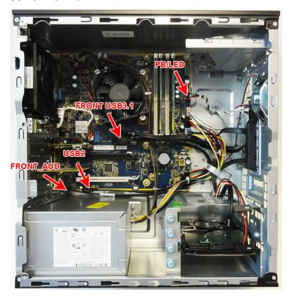
**7.** Remove the front I/O and power switch assembly from the inside of the computer.
