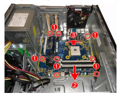
When reinstalling the system board, first insert the I/O panel back into the slots in the rear of the chassis, and then align the board with the chassis screw holes.
