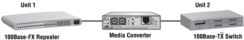
Figure 8. Example of a Duplex Mode Mismatch
