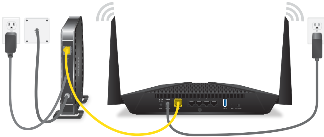
Figure 5. Cable your router
