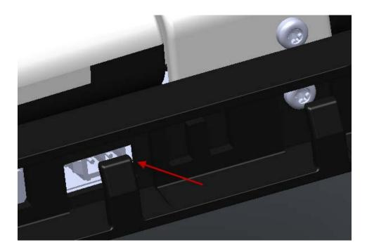
Note: Please route CMA Cable Assembly with LDS connector thru hole shown. Ensure to have enough service loop between back of unit and CMA. Route service loop to right of connector between 1U Console and CMA.
