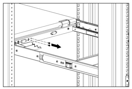
8. Attach the cable management arm to the rear of the unit with same two screws.
