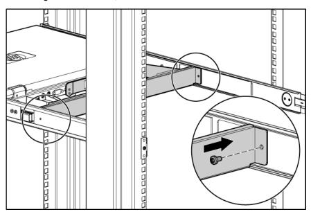
7. Remove the two screws from the rear of the unit.
