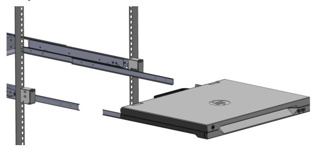
4. From the rear of the rack, slide the brace rail assembly in between the HP 1U Console Rails.
