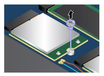
c. Carefully remove the wireless-WAN card out of the slot.
