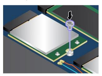
7. Connect the antenna cables to the new wireless-WAN card. Ensure that you connect the orange cable to the main connector on the card, and the blue cable to the auxiliary connector on the card.
