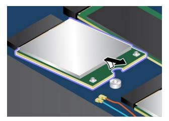
5. Align the notched edge of the new wireless-WAN card with the key in the slot. Then carefully insert the card into the slot at an angle of about 20 degrees.
