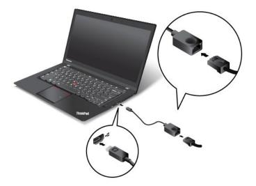
The Ethernet connector has two indicators that show the status of the network connection. When the green indicator is on, the computer is connected to a LAN. When the yellow indicator blinks, data is being transmitted.
