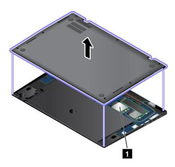
**Note:** For the user-replaceable wireless module, ensure that you use only Lenovo-authorized wireless modules for the computer. Otherwise, an error message will be displayed and the computer will beep when you turn on the computer.
