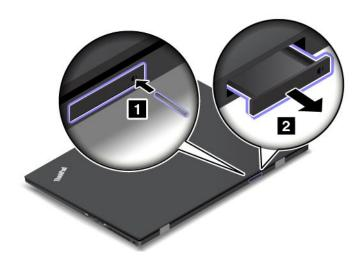
4. If you are installing a micro SIM card, go to step 5. If you are replacing a micro SIM card, gently take the old micro SIM card out of the tray first.
