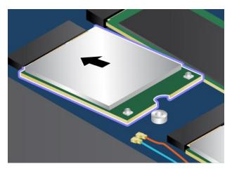
6. Install the screw to secure the card in place.
