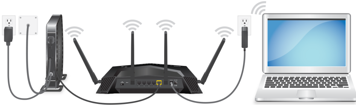
Figure 7. Cable your router
