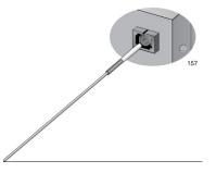
Figure 66. Cleaning a Recessed Ferrule
