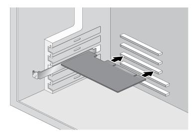
Figure 13. Inserting the Network Adapter Card
