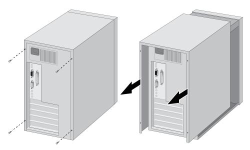
Figure 11. Removing the PC Cover
