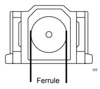
Figure 61. Ferrule in an SC Connector Plug
