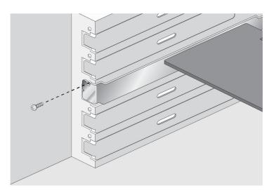
Figure 14. Securing the Adapter Card
