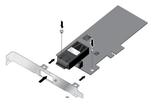
Figure 10. Fastening Screws onto Standard Bracket
