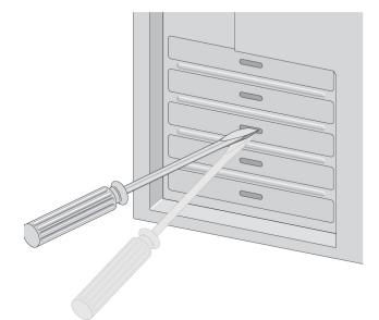
Figure 12. Removing the Faceplate From PCIe Slot
