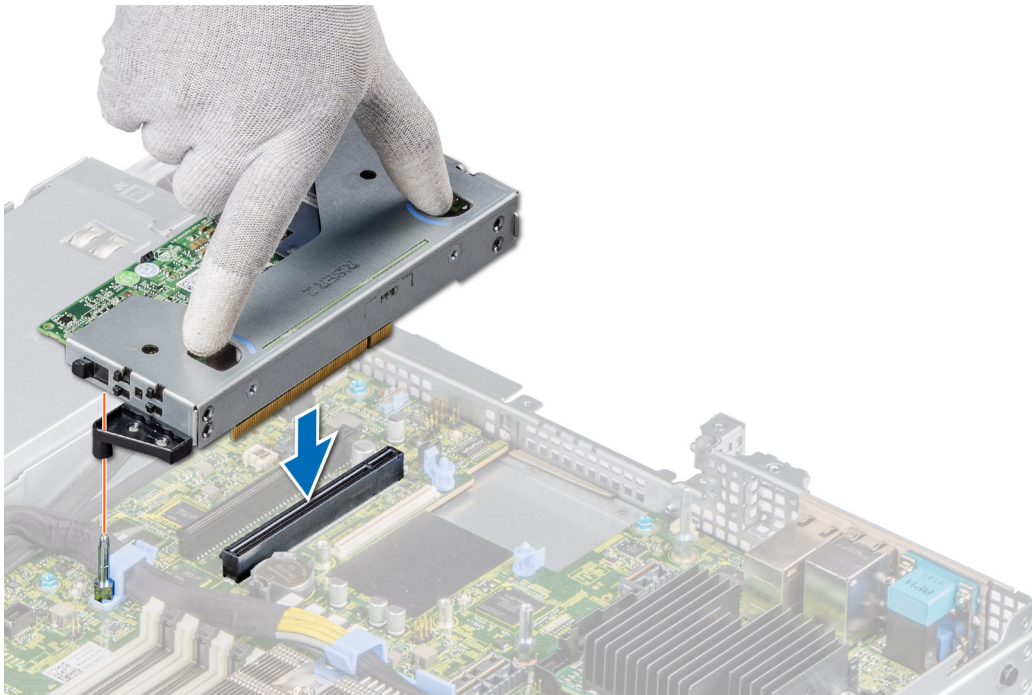
Figure 55. Installing the low profile left riser
