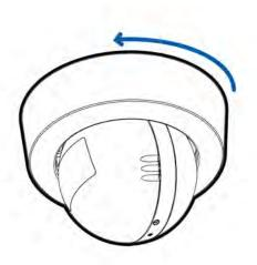
2. Pinch the camera housing clips in the attachment slots to release the camera body from the surface mount and pull the camera out of the mount.
