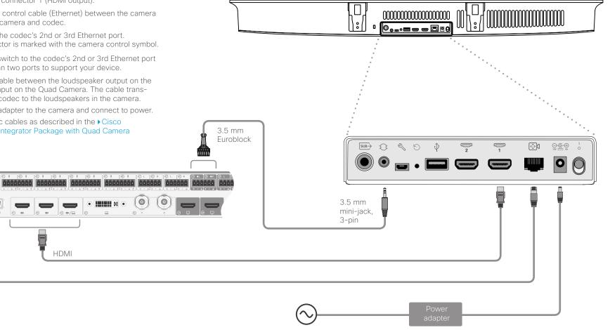
Power (100-240 V<sub>AC</sub>, 50/60 Hz) Always use the provided power cable and adapter.
