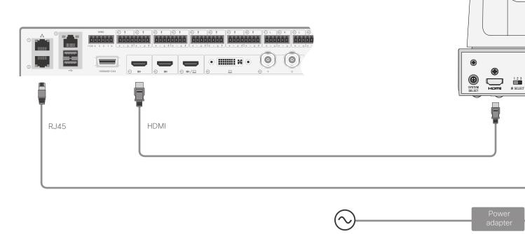
Power (100-240 V<sub>AC</sub>, 50/60 Hz) Always use the provided power cable and adapter.
