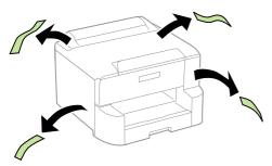
2 Open the front cover, remove all protective materials from inside the product, and close the front cover.
