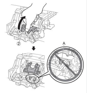
Remove the print head from the bag by holding the tab parts (A).
