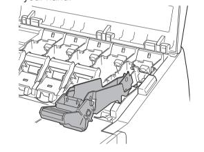
• Make sure the ink tank lock lever stays in the locked position.
