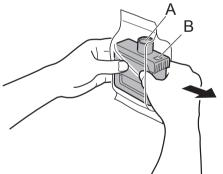
Mount the ink tank in the holder. Install with the ink holes facing down and the metal contacts facing away from you.
