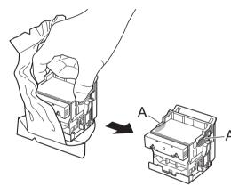
Remove the orange protective caps (A and B). Remove the protective cap (B) by holding the tab part (C).
