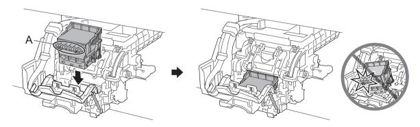
Pull the print head locking cover ③ down toward the front to lock the print head in place.
