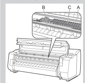
Insert the paper for adjustment between the platen (A) and paper retainer (B) in portrait orientation with the printed side of the paper facing up. Only one sheet of paper is needed.
