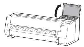
Release the ink tank lock lever for the color of ink to install. Pull the handle part (A) towards you while pressing the button at position (B).
