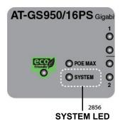
Figure 6. SYSTEM LED on AT-GS950/16PS
