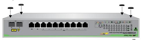
Figure 19. Attaching the Rubber Feet
