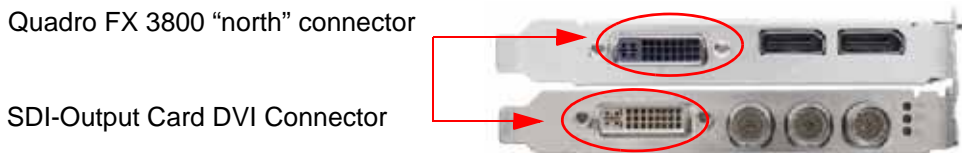
Figure 2.1 DVI Connection between the SDI Output card and the Quadro FX 3800
