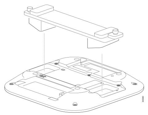
**Step 5** Screw down the thumb screws on the module.
