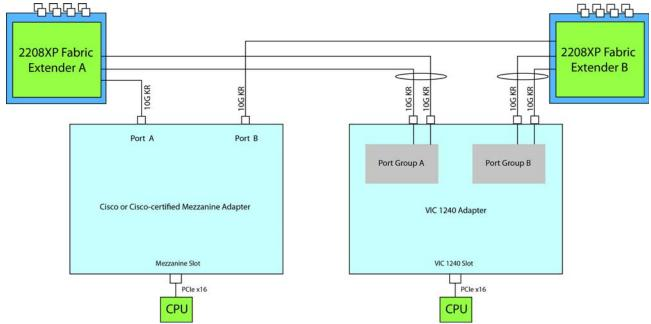
In *Figure 18*, two ports from the VIC 1240 are channeled to 2208XP Fabric Extender A and two are channeled to 2208XP Fabric Extender B. The Port Expander Card for VIC 1240 installed in the mezzanine slot acts as a pass-through device to channel two ports to each of the Fabric Extenders. The result is 40 Gbps of bandwidth to each Fabric Extender.
