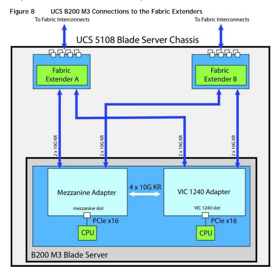
The server accommodates two types of network adapters. One is the Cisco VIC 1240 adapter. The other is a Cisco-certified I/O or flash storage mezzanine adapter. The VIC 1240 is the only adapter that can be used in the VIC 1240 slot. All other types of adapters plug into the mezzanine slot.
