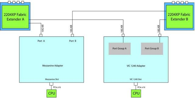
In *Figure 23*, one port from the VIC 1240 is channeled to 2204XP Fabric Extender A and one is channeled to 2204XP Fabric Extender B. The Port Expander Card for VIC 1240 installed in the mezzanine slot acts as a pass-through device to channel one port to each of the Fabric Extenders. The result is 20 Gbps of bandwidth to each Fabric Extender.
