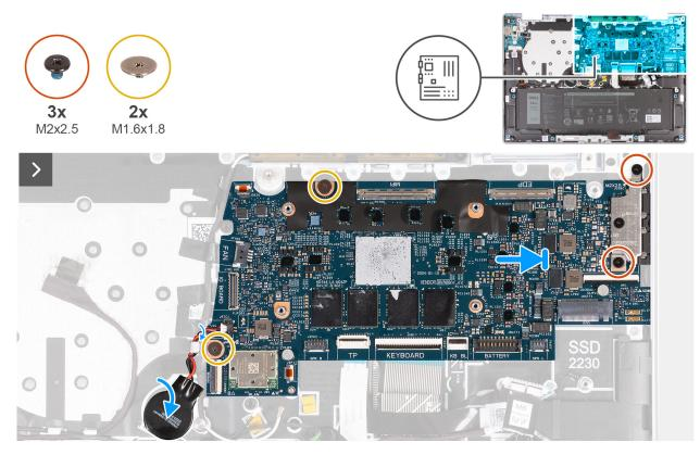
Figure 64. Installing the system board
