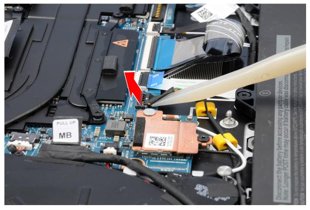
Figure 22. Prying the speaker cable from the connector
