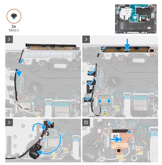
Figure 43. Installing the WLAN-antenna module
