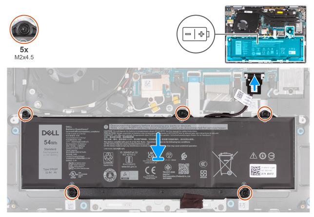
Figure 28. Installing the battery
