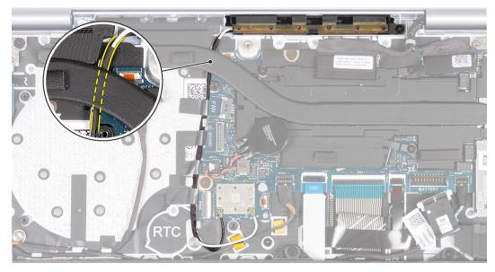
Figure 42. Removing WLAN-antenna cables
