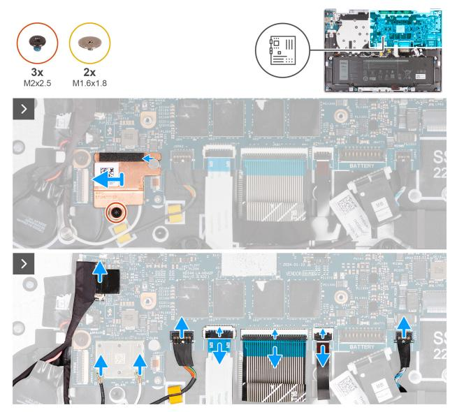
Figure 60. Removing the system board
