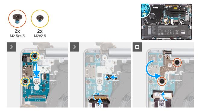
Figure 51. Installing the I/O board
