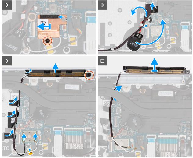
Figure 40. Removing the WLAN-antenna module
