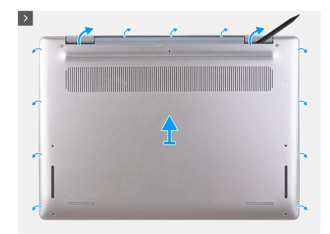
Figure 11. Removing the base cover
