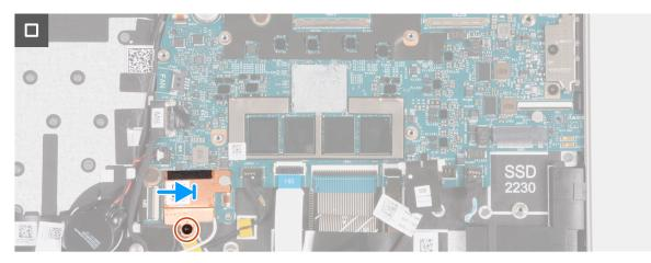
Figure 65. Installing the system board
