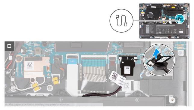
Figure 12. Disconnecting the battery cable
