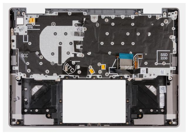
Figure 66. Palm-rest and keyboard assembly
