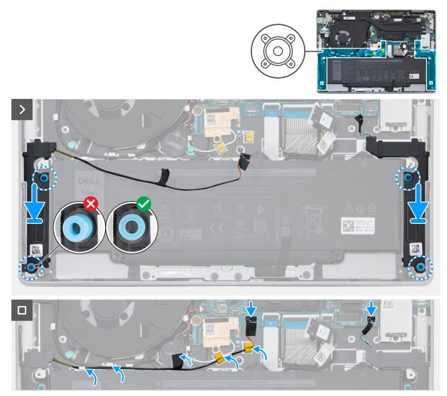
Figure 23. Installing the speakers
