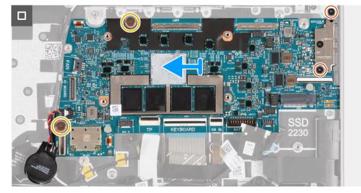
Figure 61. Removing the system board
