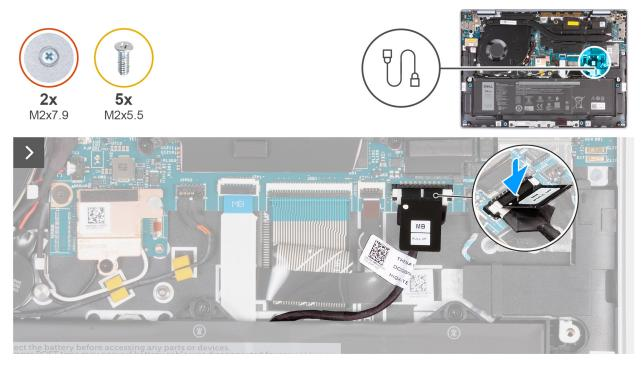
Figure 13. Connecting the battery cable
