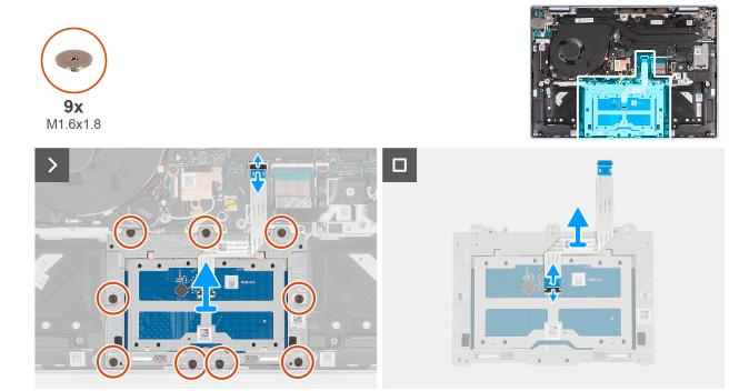
Figure 52. Removing the touchpad assembly
