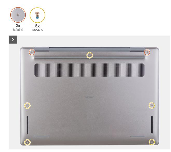
Figure 10. Removing the base cover
