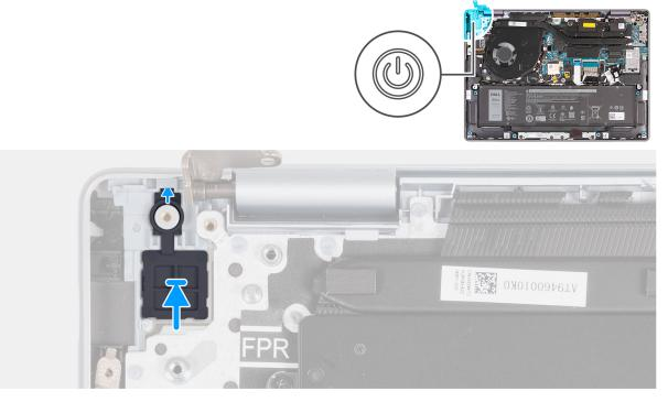
Figure 56. Installing the power button
