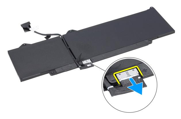
Figure 30. Disconnecting the battery cable
