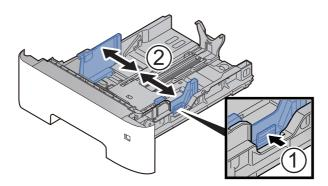
**2** Adjust the paper length guide to the paper size required. Press the paper length adjusting tab and slide the guides to the paper size required.
