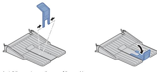
2 Install the rear tray on the rear of the machine.
