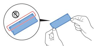
To protect electronic parts, discharge static electricity from your body by touching a water pipe (faucet) or other large metal object before handling the memory modules. Or, wear an antistatic wrist strap, if possible, when you install the memory modules.
