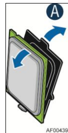
Figure 32. Installing Processor – Remove the processor protective cover
