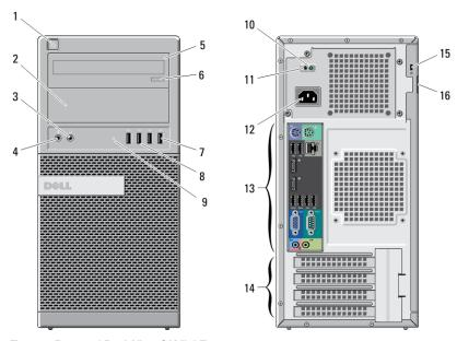
Figure 1. Front and Back View Of Mini-Tower
