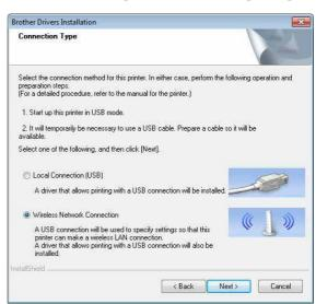
With the USB cable, connect the printer to the computer running Windows<sup>®</sup>, and then turn on the printer. If the printer is in wireless LAN mode (the WIRELESS LAN indicator is blinking), switch it to USB mode. For details, see Switching Between Wireless LAN Mode and USB Mode on page 30.
