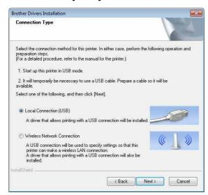
With the USB cable, connect the printer to the computer running Windows<sup>®</sup>, and then turn on the printer. Check that the printer is in USB mode (page 30), and then click [Next].
