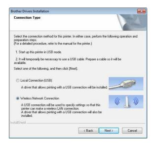
With the USB cable, connect the printer to the computer running Windows<sup>®</sup>, and then turn on the printer in USB mode. (As a factory default, the printer will be in USB mode.) If the printer is in wireless LAN mode (the WIRELESS LAN indicator is blinking), switch it to USB mode. For details, see Switching Between Wireless LAN Mode and USB Mode on page 30.
