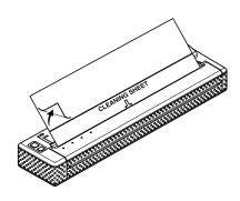
Remove the backing paper on the upper half of the cleaning sheet, as shown.
