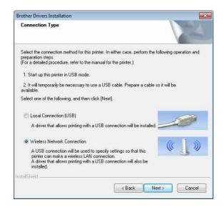
With the USB cable, connect the printer to the computer running Windows<sup>®</sup>, and then turn on the printer. If the printer is in wireless LAN mode (the WIRELESS LAN indicator is blinking), switch it to USB mode. For details, see Switching Between Wireless LAN Mode and USB Mode on page 30.
