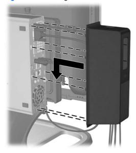
7. Slide the power supply tray out from the base of the stand (1) and place the USDT power supply into the tray (2). Route any loose cables through the cables guides on the sides of the tray (3).
