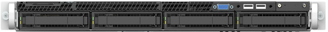
Figure 87. 3.5" Drive Bay – 4 Drive Configuration – Intel® Server System R1304WFxxxx
