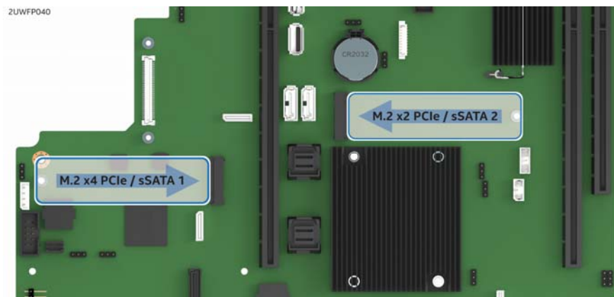
Figure 70. M.2 Connector Locations
