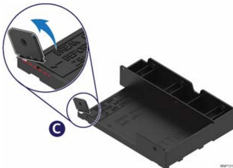
Figure 52. 3.5" Drive Carrier to 2.5" SSD Bracket – Tab Removal
