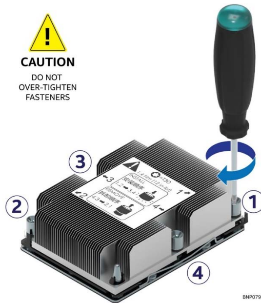
Figure 34. Installing the PHM
