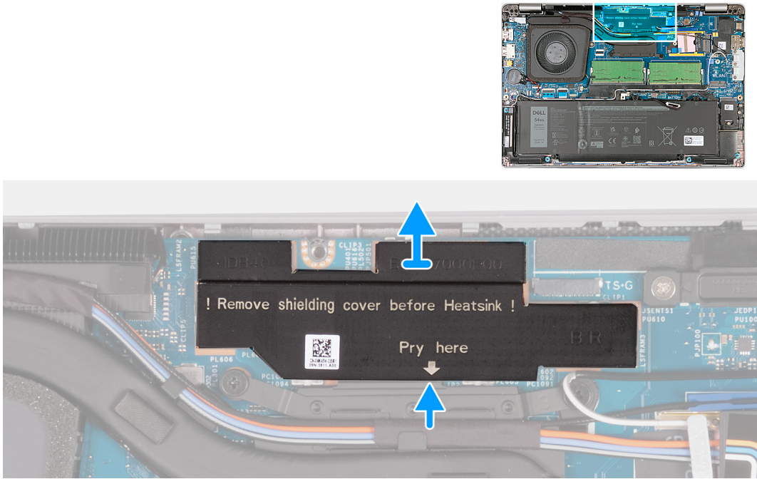
Figure 31. Removing the power shielding cover - For computers shipped with H28 UMA system board
