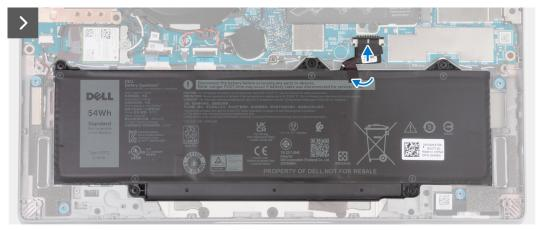
Figure 20. Connect the battery cable to the system board
