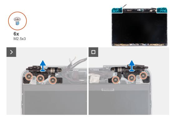
Figure 70. Removing the display hinges (laptop)
