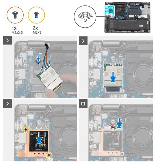
Figure 32. Installing the WWAN 5G card
