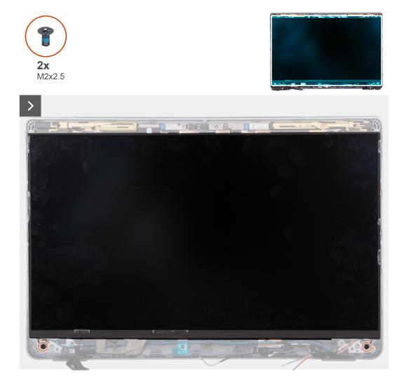
Figure 72. Removing the display panel (laptop)
