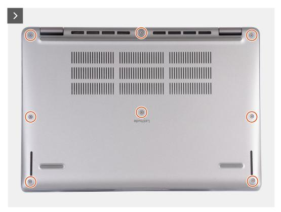
Figure 17. Loosen the eight captive screws that secure the base cover to the palm-rest assembly
