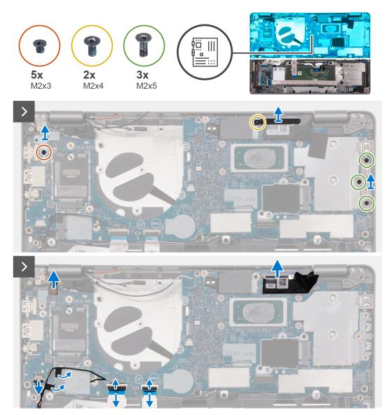
Figure 45. Removing the system board
