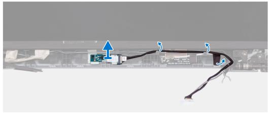
Figure 86. Removing the sensor board (laptop)
