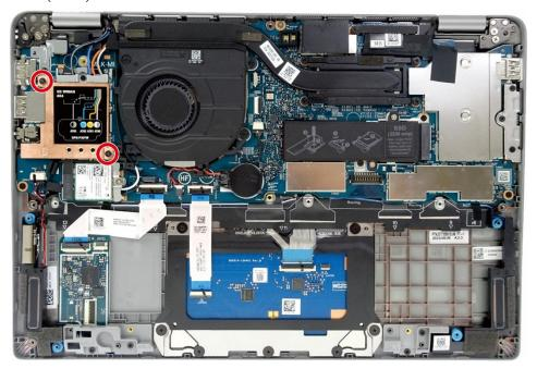
Figure 31. Metal shielding for the WWAN board
