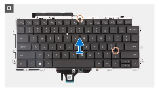
Figure 60. Removing the keyboard assembly
