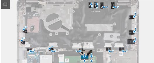
Figure 62. Installing the keyboard assembly
