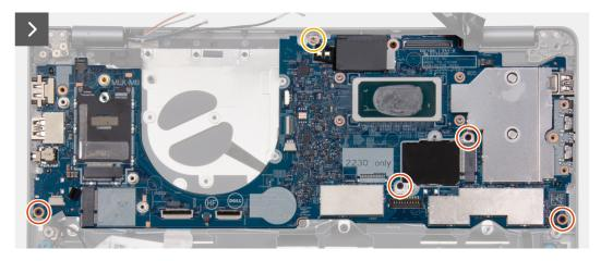
Figure 46. Removing the system board
