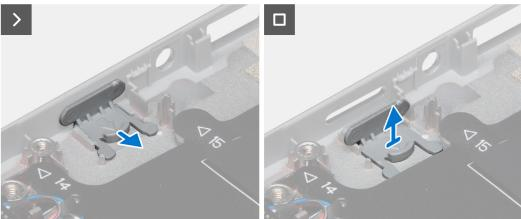
Figure 90. Removing the SIM-card slot filler
