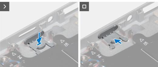
Figure 91. Installing the SIM-card slot filler
