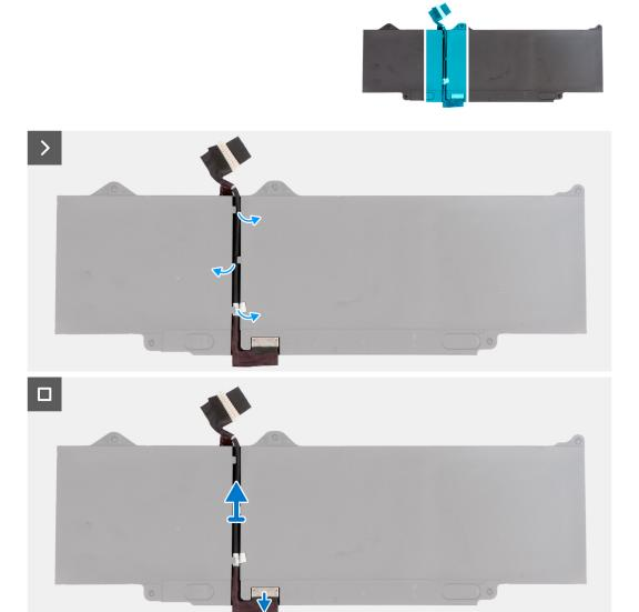
Figure 38. Removing the battery cable
