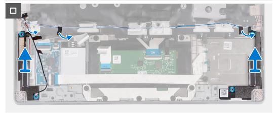
Figure 52. Removing the speakers
