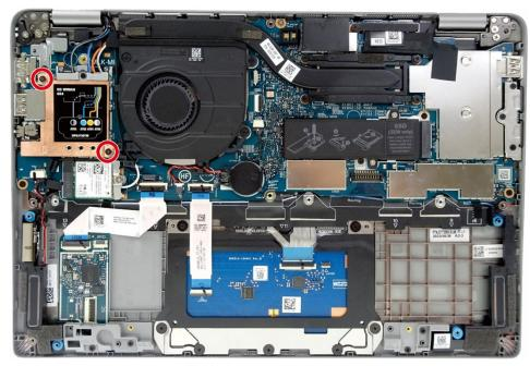
Figure 33. Metal shielding for the WWAN board
