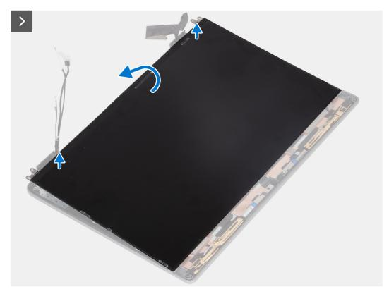
Figure 74. Removing the display panel (laptop)
