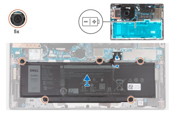
Figure 36. Removing the battery
