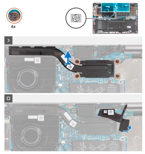
Figure 43. Installing the heat sink
