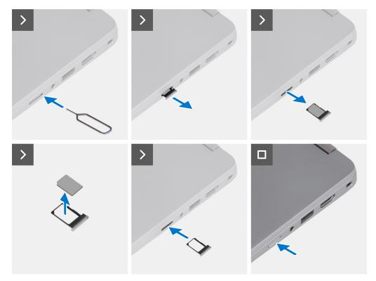
Figure 15. Removing the SIM card tray
