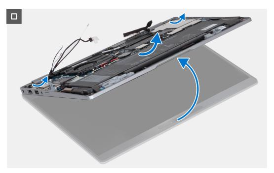
Figure 64. Removing the display assembly
