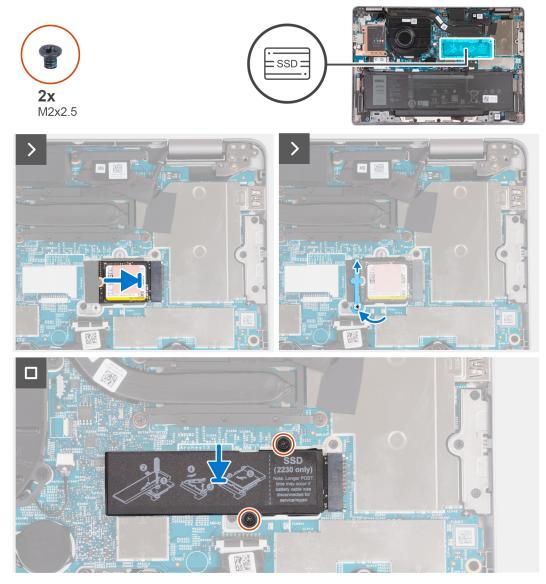
Figure 24. Installing the M.2 2230 SSD
