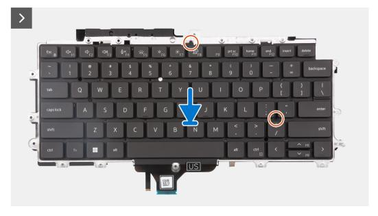
Figure 61. Installing the keyboard assembly
