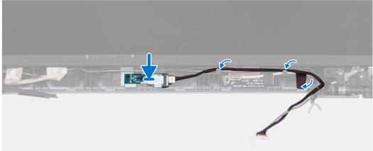
Figure 87. Installing the sensor board (laptop)
