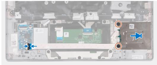
Figure 89. Installing the smart-card reader
