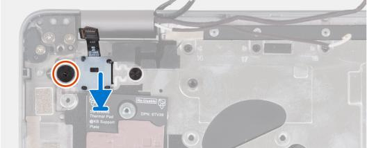
Figure 58. Installing the power button with fingerprint reader
