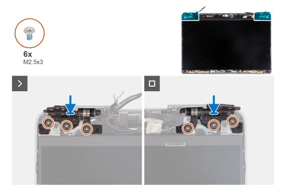
Figure 71. Removing the display hinges (laptop)
