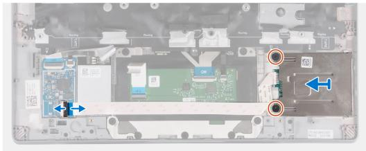
Figure 88. Removing the smart-card reader
