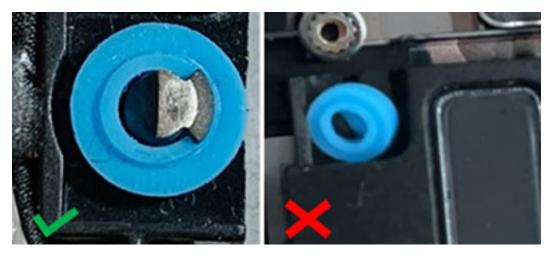
Figure 54. Rubber grommets of speaker
