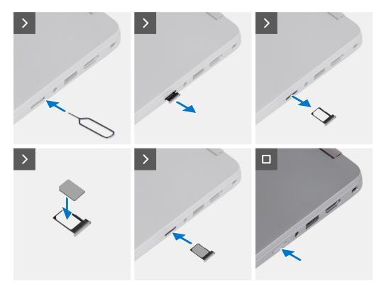
Figure 16. Installing the SIM card tray
