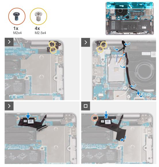
Figure 66. Installing the display assembly
