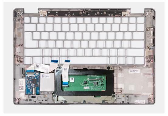
Figure 92. Removing the palm rest
