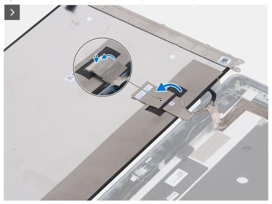
Figure 77. Installing the display panel (laptop)
