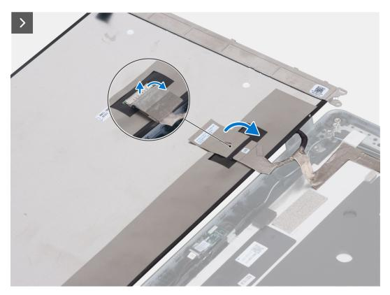
Figure 75. Removing the display panel (laptop)
