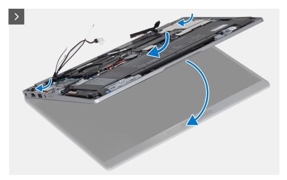
Figure 65. Installing the display assembly
