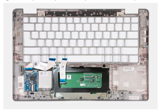
Figure 93. Installing the palm rest
