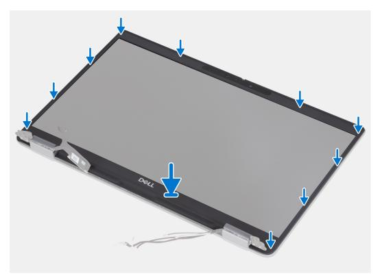
Figure 69. Installing the display bezel (laptop)
