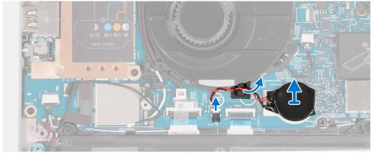
Figure 40. Removing the coin-cell battery
