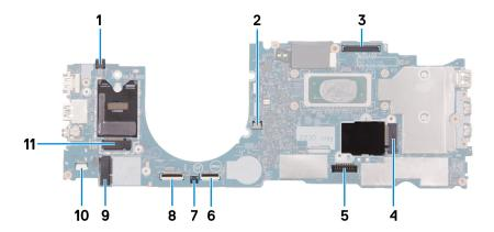
Figure 48. System-board connectors
