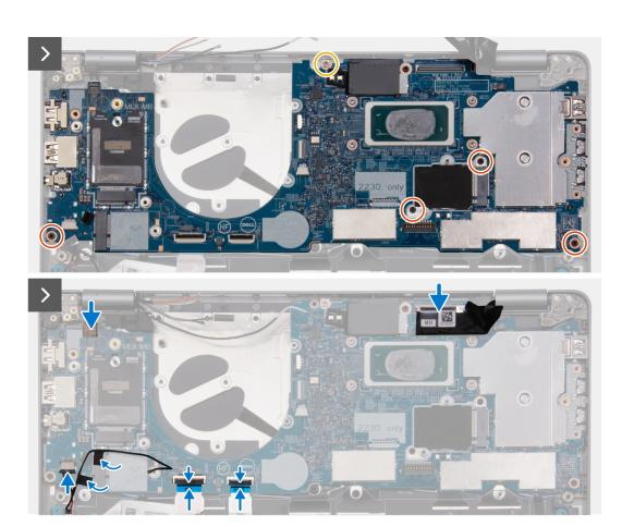
Figure 50. Installing the system board
