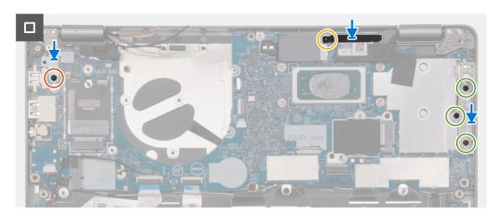
Figure 51. Installing the system board
