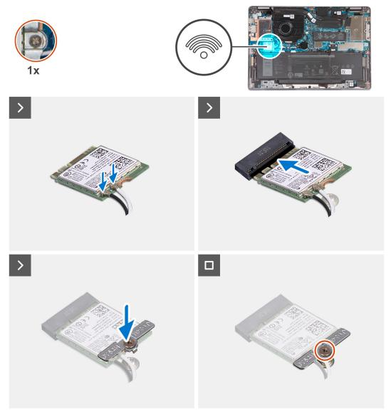
Figure 26. Installing the wireless card
