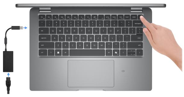
Figure 12. Connect the power adapter and press the power button
