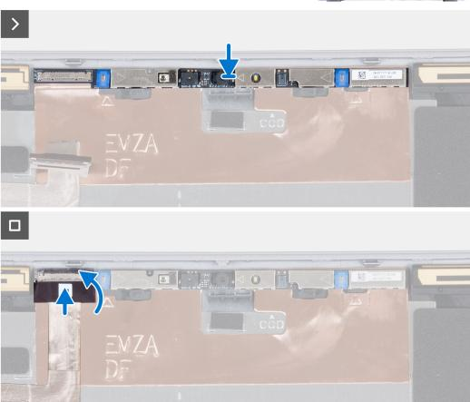
Figure 83. Installing the camera (laptop)
