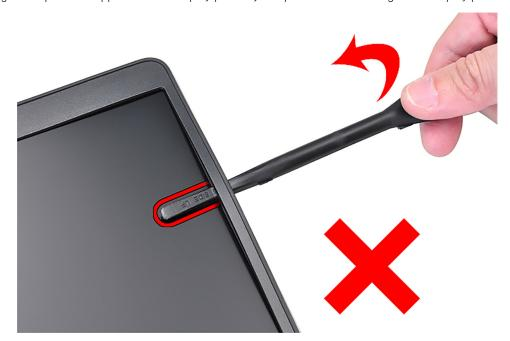
Figure 68. Prying the display bezel (laptop)
