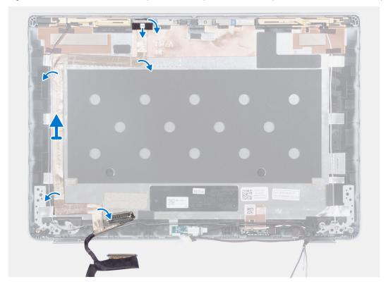
Figure 80. Removing the display cable (laptop)
