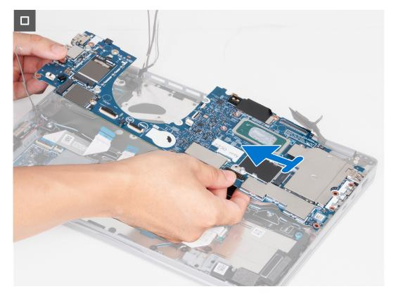
Figure 47. Removing the system board
