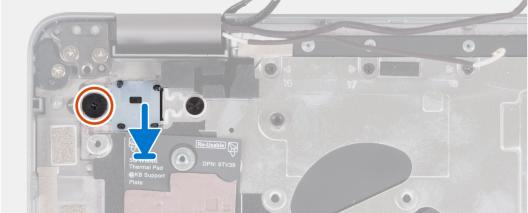
Figure 56. Installing the power button
