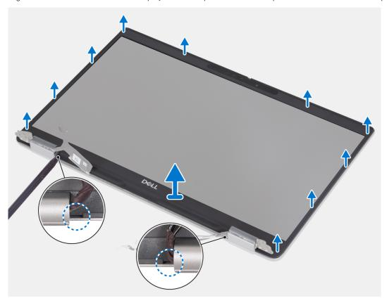
Figure 67. Removing the display bezel (laptop)
