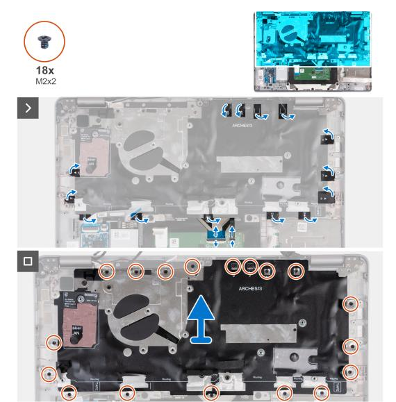
Figure 59. Removing the keyboard assembly
