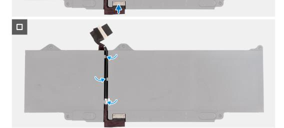
Figure 39. Installing the battery cable
