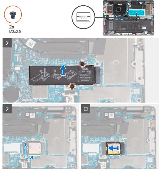
Figure 23. Remove the M.2 2230 SSD
