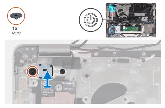
Figure 55. Removing the power button
