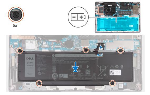
Figure 37. Installing the battery
