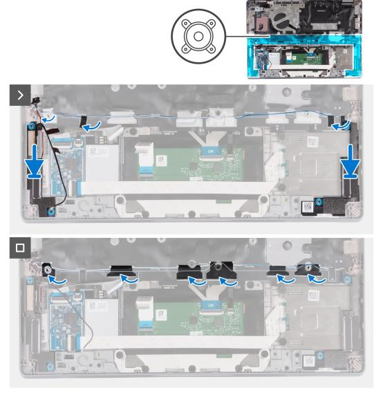
Figure 53. Installing the speakers
