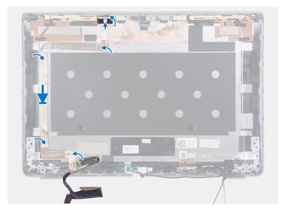
Figure 81. Installing the display cable (laptop)
