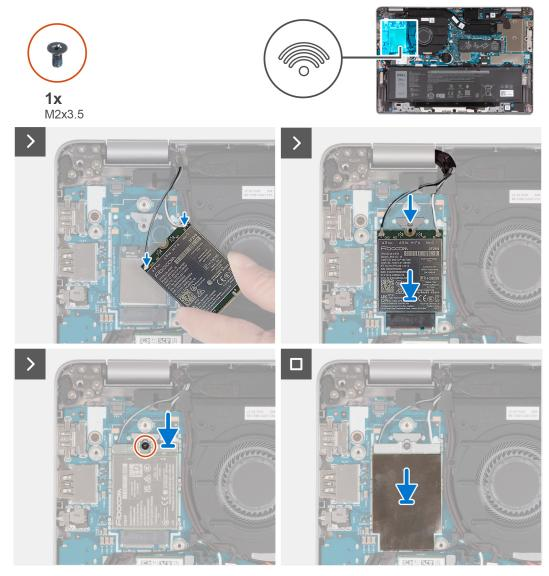
Figure 29. Install the WWAN 4G card
