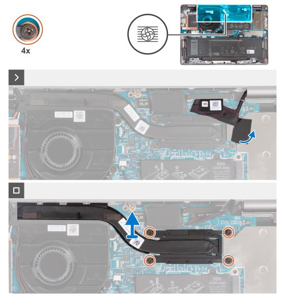
Figure 42. Removing the heat sink
