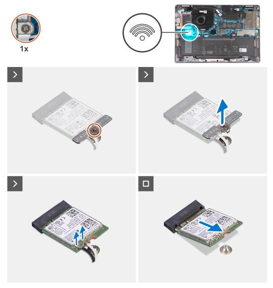
Figure 25. Remove the wireless card
