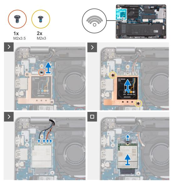
Figure 30. Removing the WWAN 5G card
