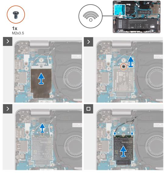
Figure 28. Remove the WWAN 4G card
