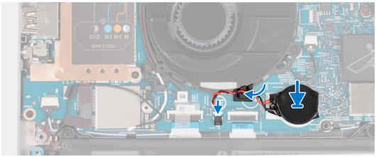
Figure 41. Installing the coin-cell battery
