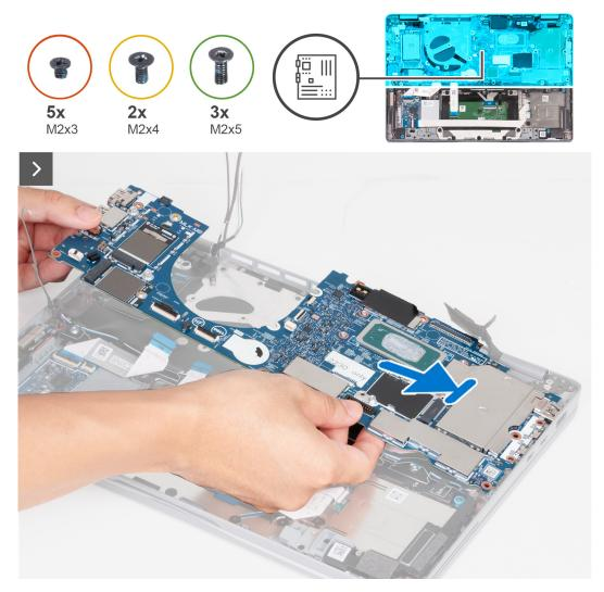
Figure 49. Installing the system board
