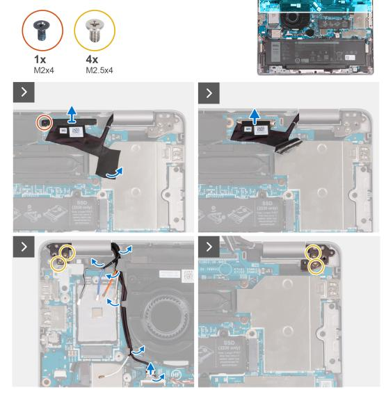
Figure 63. Removing the display assembly
