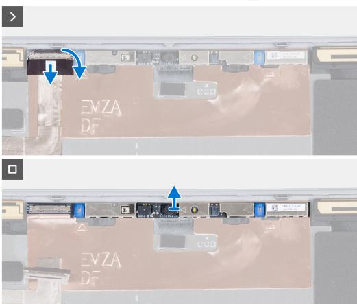
Figure 82. Removing the camera (laptop)
